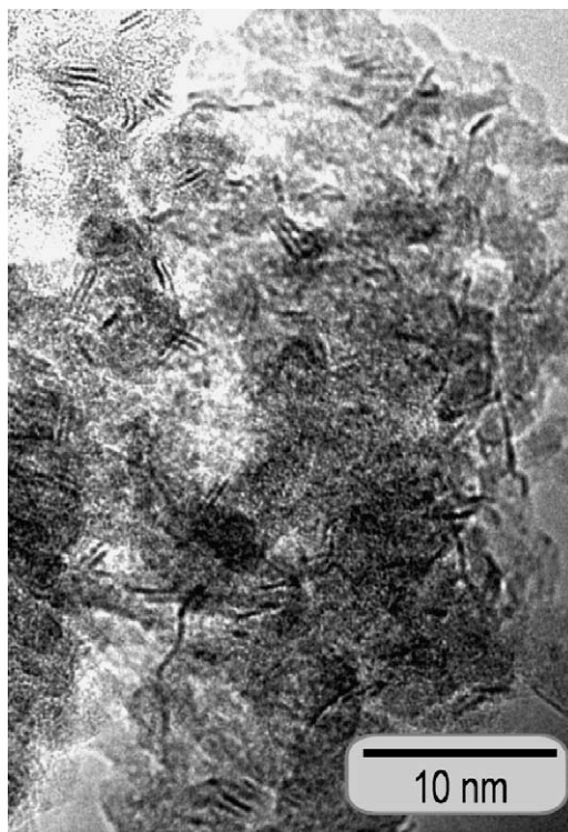
Fig. 7. TEM image of NiW/ASA-673 after sulfidation at 673 K showing single- and multiple-layered slabs representative for the largest part of the sample.
